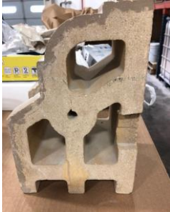
Side view of terra cotta unit showing webbing
