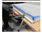
**6.** The mix will begin to set within 1 hour. If you added a wire mesh, now is the time to snip off the wire ties holding the mesh. Cover the countertop mix with plastic and allow it to cure for 18-24 hours in dry conditions.
