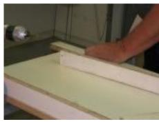
**1.** Build a form for making your countertop using  $\frac{3}{4}$ " Melamine coated particleboard. Cut strips for the sides 1  $\frac{1}{2}$ " – 3" wide to match the desired countertop thickness.
