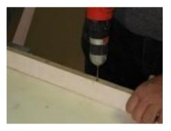
**2**. Drill guide holes on the side boards from the top down and assemble the side panels to the bottom panel using 2" coarse drywall screws. Fasten the sides of the form to the base using coarse screws allowing for the depth of the countertop and fastening securely to the base. Fasteners should be located ever 6-8 inches are the perimeter.
