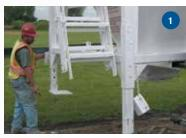
A DOUBLE BATCH OF MATERIAL IS MADE IN 5 MINUTES OR LESS WITHOUT STRAINING THE LABORERS OR COMPROMISING THE INTEGRITY OF THE MIX. NO ELECTRICITY OR PRESSURIZED WATER SOURCE IS NEEDED FOR THE TEN BAGGER, JUST A STANDARD MECHANICAL BATCH MIXER. THE SILO IS TRANSPORTABLE. AS THE JOB PROGRESSES, THE CREW AND TEN BAGGER MIXING STATION FOLLOW. THIS IS HOW IT WORKS:
