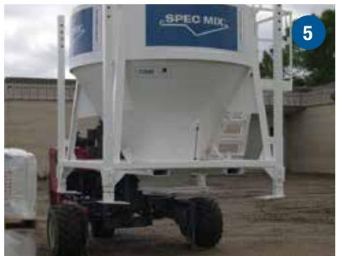
**Step 5:** The silo is easily relocated on site to position your mixing station as close as possible to the work, maximizing job site efficiency. With the silo legs pinned in the up or down position, insert the forks of the lift into the silo's fork pockets. Then, raise the silo and place it in the preferred location. Make sure the forklift is equipped to safely transport the silo and that the new terrain is dry, level and stable. Always secure all leg pins and safety pins!
