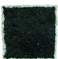
8% active content 60 second exposure 1–2mm (1/16") active penetration ~4–8 years normal weather protection\*
