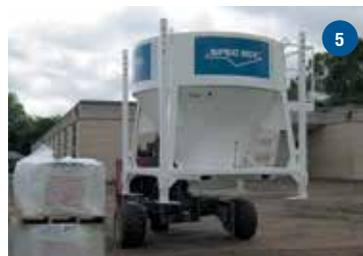
A DOUBLE BATCH OF MATERIAL IS MADE IN 5 MINUTES OR LESS WITHOUT STRAINING THE LABORERS OR COMPROMISING THE INTEGRITY OF THE MIX. NO ELECTRICITY OR PRESSURIZED WATER SOURCE IS NEEDED FOR THE TEN BAGGER, JUST A STANDARD MECHANICAL BATCH MIXER. THE SILO IS TRANSPORTABLE. AS THE JOB PROGRESSES, THE CREW AND TEN BAGGER MIXING STATION FOLLOW. THIS IS HOW IT WORKS:
