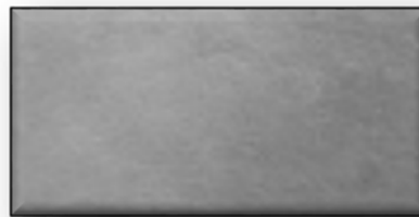
CSP 1 (acid etched)
